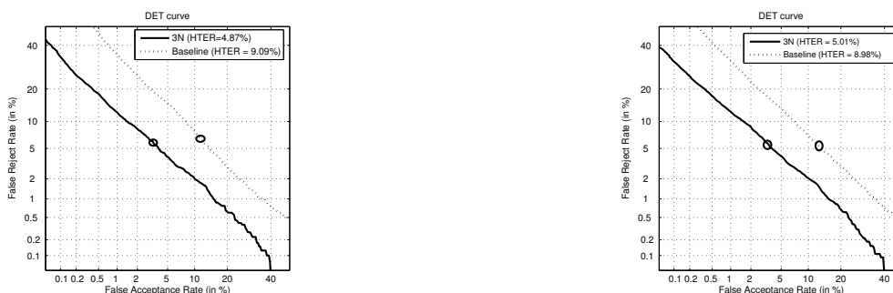
Figure 2: DET curves obtained for the baseline system (dotted line) and 3N normalization (continuous line) for the male MOBIO evaluation dataset (left) and full MOBIO dataset (right), and the HTER operating point (circle).
