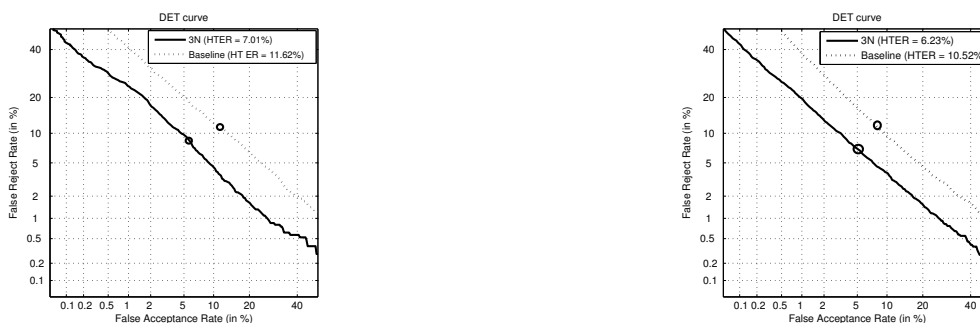
Figure 1: DET curves obtained for the baseline system (dotted line) and 3N normalization (continuous line) for the female MOBIO evaluation dataset (left) and full MOBIO dataset (right), and the HTER operating point (circle).
