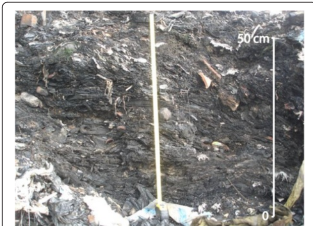
Figure 6 Internal structure of the deposit showing undulating discontinuities and foliated layers (photo: P. Wassmer, February 2007).
