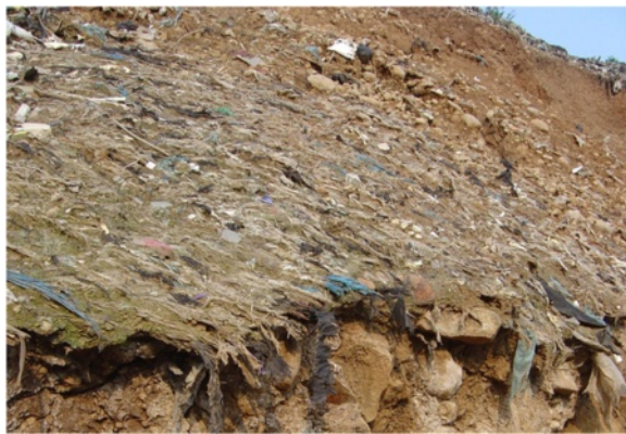
Figure 7 Pieces of plastic bags displaying horizontal orientations along the post-disaster scarp of the dump (Photo: F. Lavigne, July 2005).
