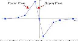
Figure 7. Non-linear force/distance profile for a plucking interaction
