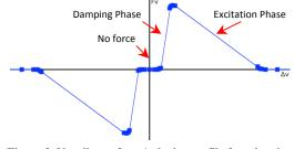
Figure 9. Non-linear force/velocity profile for a bowing interaction
