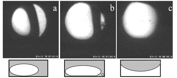
FIG. 4: Heater drying dynamics at the CHF at  $T = 32.5\text{K}$  visualized through the transparent heater (closest to the observer). (a) Initial bubble position at equilibrium. (b) Bubble partially spread. (c) The heater is completely dried out. The section of the cell interior with a plane perpendicular to the image is sketched below the corresponding photo. On the sketches, the vapor is white and the liquid is gray; the heater is at the bottom.
