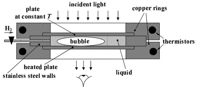
FIG. 2: Sketch of the cylindrical transparent experimental cell.
