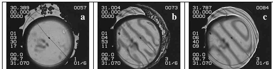
Figure 8. Shown are some of the events that occurred in the final portion of a ramp similar to the ramps shown in Figure 3 in a cell filled with \text{CO}_2 . This cell contains 3 thermistors and a piston to vary the fluid density between ramps. In this case the fluid was at \delta\rho = -3.5\% below the critical density. Figure 8a shows that a cluster of bubbles has formed at the edge of the cell far below T_C . One of these bubbles has coalesced with the large bubble producing a hot plume that travels toward the center of the large bubble. Figure 8b, at approximately T_C , shows a
