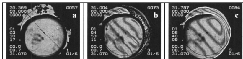
FIG. 8. Shown are some of the events that occurred in the final portion of a ramp similar to the ramps shown in Fig. 3 in a cell filled with CO 2 . This cell contains three thermistors and a piston to vary the fluid density between ramps. In this case the fluid was at \delta\rho = -3.5\% below the critical density. Panel (a) shows that a cluster of bubbles has formed at the edge of the cell far below T_C . One of these bubbles has coalesced with the large bubble producing a hot plume that travels toward the center of the large bubble. Panel (b), at approximately T_C , shows a considerably distorted grid shadow image with critical opalescence at the sidewall in the region just where the bubbles were nucleating. The dynamical activity suddenly stops at about the same time as this layer forms. The particular phase distribution that existed just before the critical temperature was passed appears to be frozen in place. The image in panel (c) is above the critical temperature T_C and the grid shadows in this image shows significant density changes. Slower mass fluxes continue, however, and the system evolves to a uniform supercritical fluid not long after panel (c).
