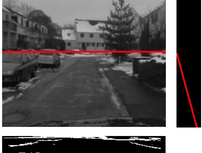
Figure 2: Left top: Original left image with calculated horizon line in red; Right top: V-disparity map with calculated ground plane line; Bottom: U-disparity map
