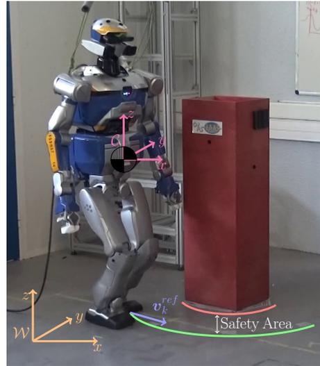
Fig. 1: HRP-2 avoiding reactively on an obstacle, even if the reference velocity  $v_k^{ref}$  drives it into it. The upper body geometry is taken into account by setting a constraint (in green) such that the robot is sufficiently away from the obstacle (in red).
