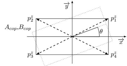
Fig. 4: Shape of the foot with the position vector  $p_i^z$  describing the support polygon and  $\theta$  representing its orientation. The  $4 \times 2$  matrix  $A_{cop}$  and the  $4 \times 1$  vector  $B_{cop}$  are the linear algebra representation of the edges.
