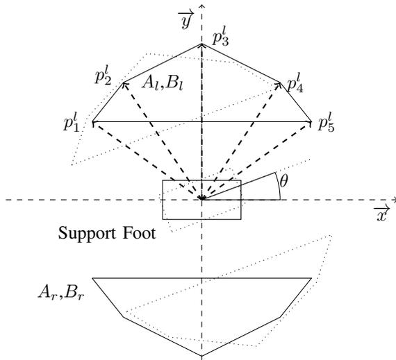
Fig. 5: Shape of the selected convex polygon boundary of the foot placement. The  $5 \times 2$  matrix  $A_{rl}$  and the  $5 \times 1$  vector  $B_{rl}$ , define the convex hull as a set of linear inequalities.
