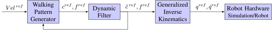
Fig. 3: The control scheme:  $Vel^{ref}$  is the input velocity.  $c^{ref}$  and  $f^{ref}$  are respectively the CoM and the feet 3D trajectories  $\tilde{c}^{ref}$  is the CoM trajectory filtered.  $q^{ref}$ ,  $\dot{q}^{ref}$  denote respectively the generalized coordinate vector and its derivation.
