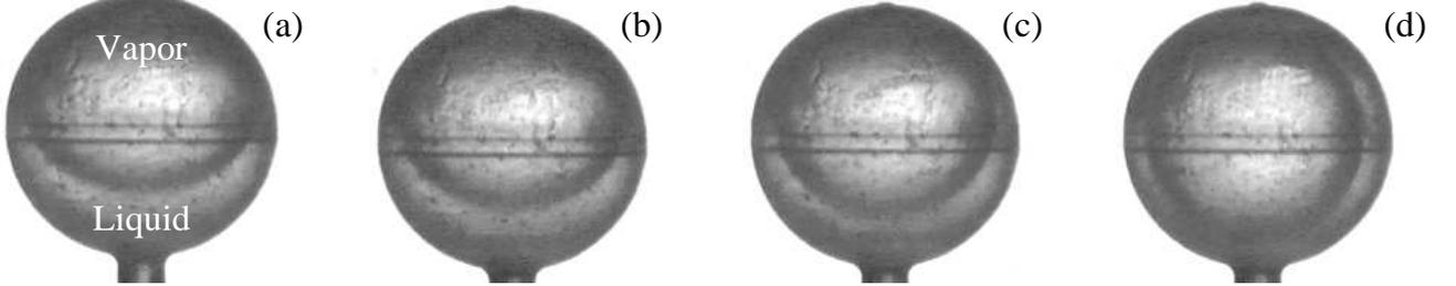
Fig. 5. The sphere half filled with liquid hydrogen at a temperature close to the triple point (14 K) for the different values of the current  $I$  in the solenoid that correspond to the different amplitudes of the magnetic field: (a)  $I = 0$ , (b)  $I = 30$  A, (c)  $I = 50$  A, (d)  $I = 60$  A. The gravity is completely compensated by the magnetic force. The gas bubble is stable and well centered.
