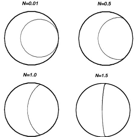
FIG. 12: Calculated bubble shape for different values of the non-dimensional strength of vapor recoil  $N$  that goes to infinity at the critical point. Note that the actual contact angle is zero for all the curves.
