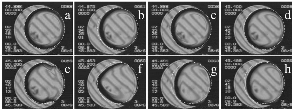
FIG. 10: Time sequence of images of cell 8 during two 100 mK quenches. The gas spreads during each quench that lasts about 12 s. The equilibrium position of the vapor bubble with respect to the cell is shown by the white circle in each image for comparison.
