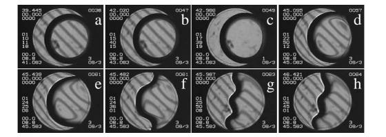
FIG. 8: Time sequence of the images from cell 8 during continuous heating through the critical point. Images (a-h) were taken exactly for the same values of temperature (shown in Fig. 5) as corresponding images in Fig. 6. The magnified upper regions close to the contact line from the images (e-h) are shown in Fig. 7.
