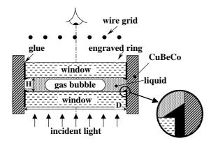
FIG. 1: Sketch of a cross-section of the cylindrical sample cell (with parallel windows). The fluid volume is contained between two sapphire windows that are glued to a CuBeCo alloy ring. The dimensions H (see Table I) and D(=12 mm) of the cell are indicated. Some glue is squeezed into the cell. The thickness of the glue layer is exaggerated for illustration purposes. In weightlessness, the gas bubble should be located in the middle of such an 'ideal' cell, see sec. III for the discussion.
