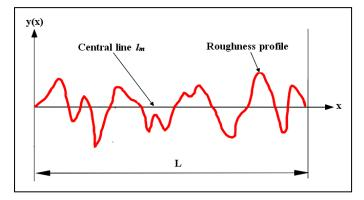
Fig. 2. Roughness profile characteristics.
