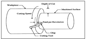
Fig. 1. Basic turning operation.
