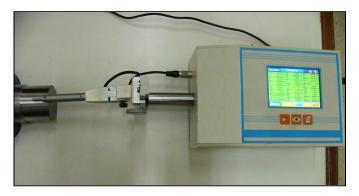
Fig. 5. Measurement of surface roughness by Roughness Tester.
