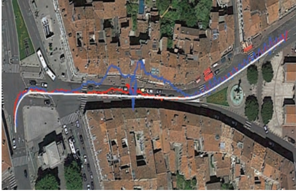
Fig. 7. Positioning results for different approaches in a urban canyon (obtained with Google Earth). Reference trajectory: white line; proposed approach: red line; standard EKF: blue line. (For interpretation of the references to color in this figure caption, the reader is referred to the web version of this paper.)
