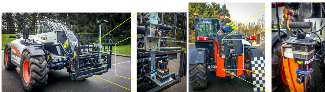
Figure 2. The telescopic forklift Bobcat TL470: Real images of the acquisition system setup in two different configurations.
