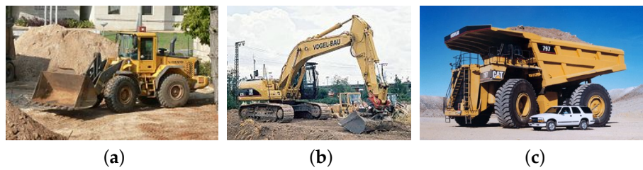
Figure 1. Common types of heavy machines. (a) Loader; (b) excavator; (c) truck.
