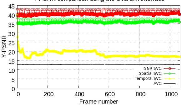
Y-PSNR comparison using the OverSim interface
