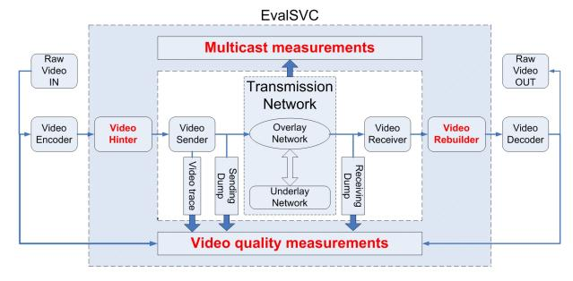
Fig. 9. EvalSVC and the performance evaluation of different types of SVC transmission on overlay network.
