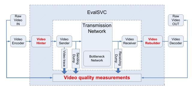
Fig. 4. EvalSVC with the evaluation of the SVC transmission on bottleneck network.
