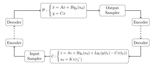
Figure 1: Feedback loop where the inputs and outputs are time-sampled and quantized.
