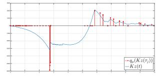
(a) The plot contains the continuous-time signal  $\tilde{y}$  (continu- (b) Plot of the continuous-time control input with its spaceous curve in blue) with its space-quantized and time-sampled values transmitted to the controller (dots in red color). The quantization parameter  $\nu$  converges to zero very quickly, and hence a very little difference is observed between the quantized and real values.
