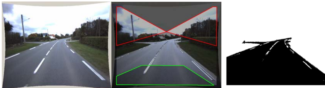
Figure 3 : The original image of the front road on the left is processed learning road colors from pixel colors of the green region, and learning non-road colors from the red ones. The result of the classification of the pixels in road and non-road pixels is shown on the right.
