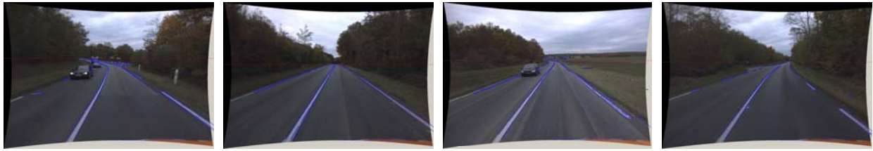
Figure 5 : The blue edges are the edges of the right image registered on the left image, which is displayed. These images are extracted from a sequence of 400 images from road RD372, CG 91.
