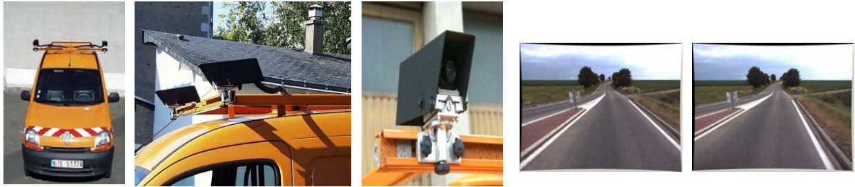
Figure 1 : Experimental inspection vehicle with two digital cameras for stereovision (left 3 images, by courtesy of CECP). On the rightmost part of the figure, a stereo pair of images acquired by the vehicle is displayed.
