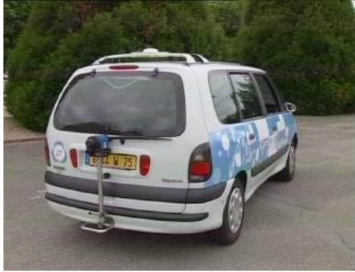
Figure 1: The instrumented vehicle and laser scanner
