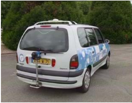
Figure 1. The instrumented vehicle and laser scanner
