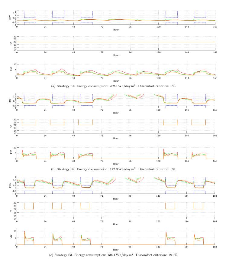
Figure 13: Results from July 6 to July 12, 2011 (cooling mode), using strategies S1 (a), S2 (b) and S3 (c).  $PMV_j$  (top),  $T_j^{sp}$  (middle) and  $P_j$  (bottom),  $\forall j \in [\
