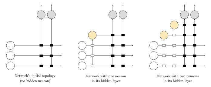
Figure 3: The cascade-correlation algorithm. White, beige and grey circles deal with inputs, hidden neurons and output neurons, respectively. Black rectangles depict weighted connections between inputs and output neurons or between hidden neurons and output neurons. White rectangles depict weighted connections between inputs and hidden neurons or between hidden neurons.
