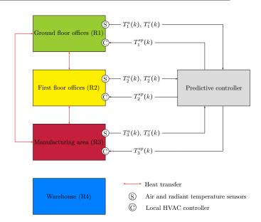
Figure 2: The three rooms in the building (R1, R2 and R3) equipped with air and radiant temperature sensors ( $T_j^a$  and  $T_j^r$ ,  $\forall j \in \llbracket 1; 3 \rrbracket$ ) and controlled HVAC subsystems. The warehouse (R4) is unheated. No heat transfer between the warehouse and the other rooms of the building is explicitly taken into account.  $T_j^{sp}$ ,  $\forall j \in \llbracket 1; 3 \rrbracket$ , is the HVAC temperature set-point in the room j.
