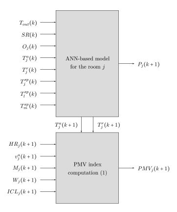
Figure 4: ANN-based model for the room j,  $\forall j, l, m \in [1; 3]$  such as  $j \neq l \neq m$ .  $PMV_j$  is computed at time step k+1 using (1) (Section 3, heating or cooling mode).
