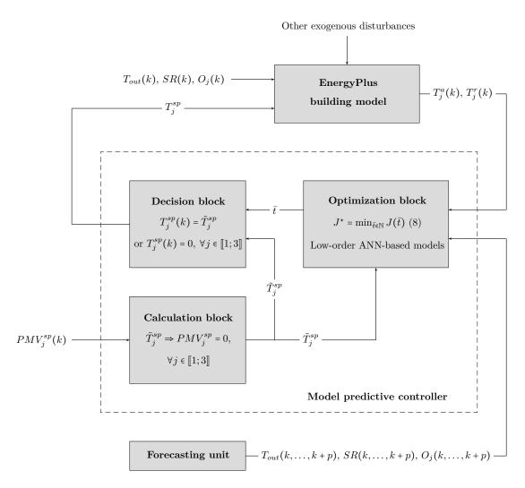
Figure 5: Block diagram of the predictive control strategy. See Sections 3 and 4 for a description of the parameters involved in the strategy.
