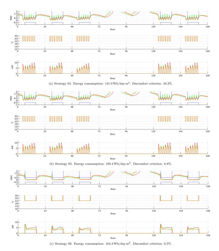
Figure 14: Results from July 6 to July 12, 2011 (cooling mode), using strategies S4 (a), S5 (b) and S6 (c).  $PMV_j$  (top),  $T_j^{sp}$  (middle) and  $P_j$  (bottom),  $\forall j \in [\
