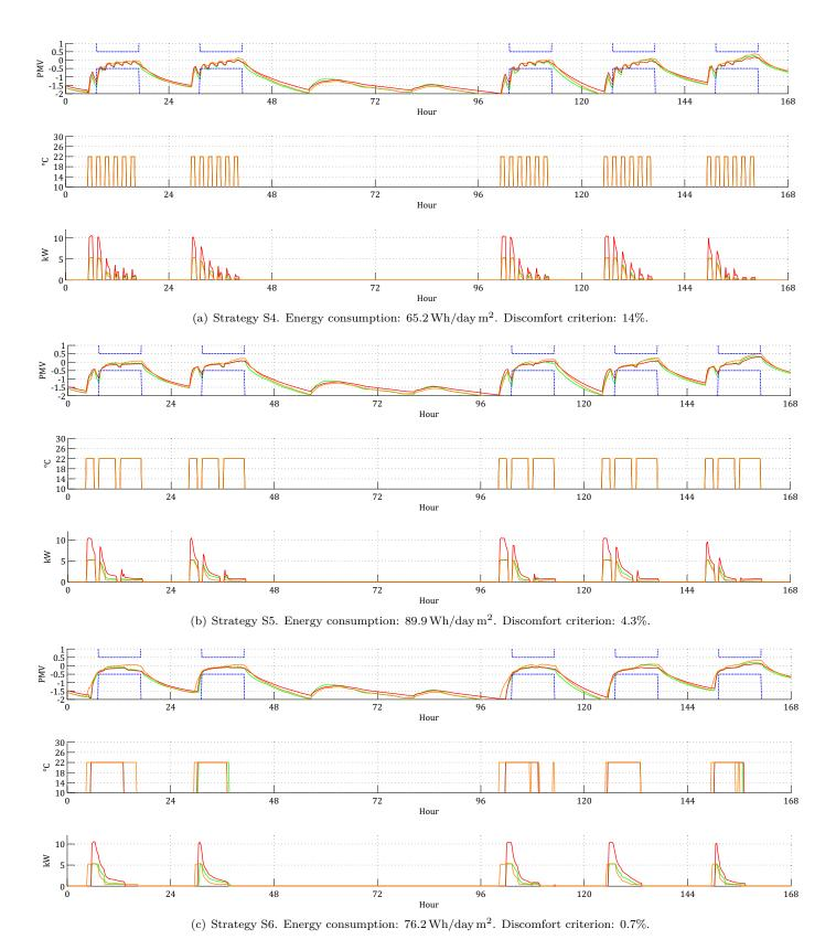
Figure 12: Results from January 6 to January 12, 2011 (heating mode), using strategies S4 (a), S5 (b) and S6 (c).  $PMV_j$  (top),  $T_j^{sp}$  (middle) and  $P_j$  (bottom),  $\forall j \in [1;3]$ . Green color is for the ground floor offices, orange color is for the first floor offices and red color is for the manufacturing area. Blue color is for  $PMV_j^{min}$  and  $PMV_j^{max}$ .
