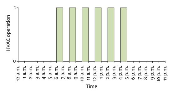
Figure 9: Daily HVAC operation (S4). 0 is for non-operating HVAC subsystems, 1 is for subsystems in operation.
