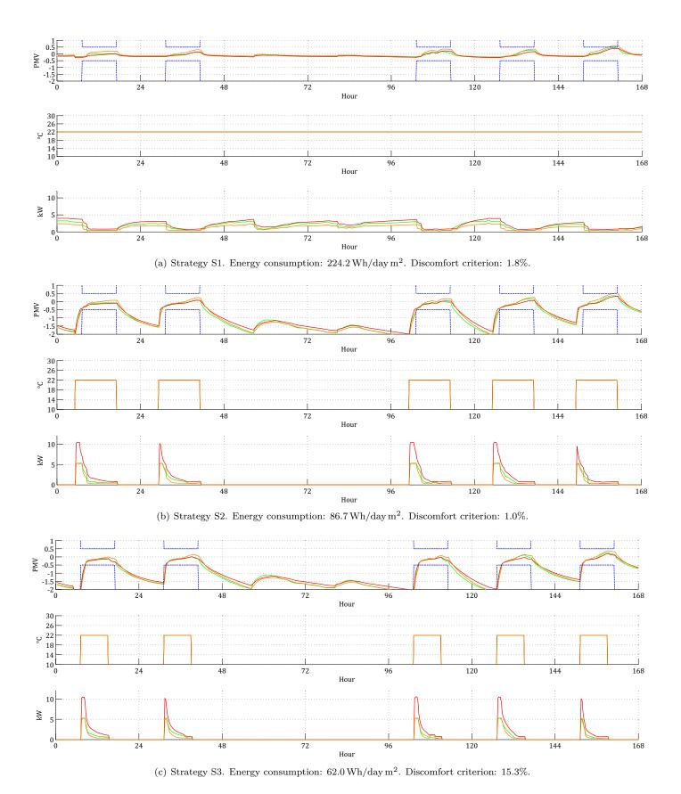
Figure 11: Results from January 6 to January 12, 2011 (heating mode), using strategies S1 (a), S2 (b) and S3 (c).  $PMV_j$  (top),  $T_j^{sp}$  (middle) and  $P_j$  (bottom),  $\forall j \in [\
