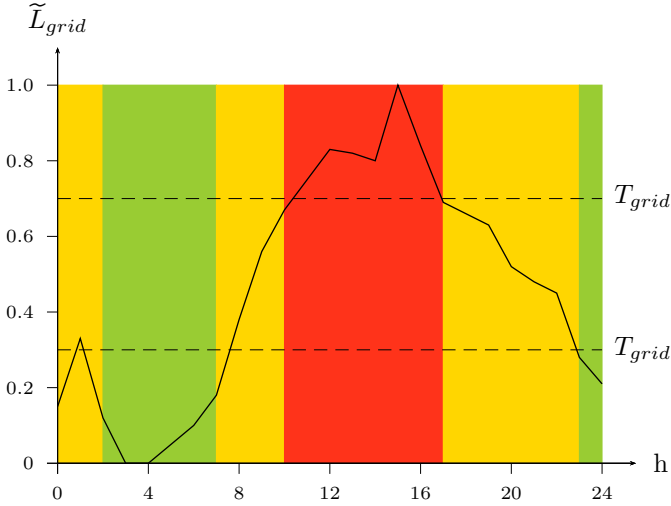
Figure 7: Normalized daily load of the “Perpignan-Méditerranée” agglomeration community ( \tilde{L}_{grid} ) during the “summer/autumn” season ( i.e. May 1 to October 31). Red, yellow and green colors are for on-peak, part-peak and off-peak periods, respectively. Dashed lines are for the grid thresholds ( T_{grid} = 30\% and T_{grid} = 70\% ).
