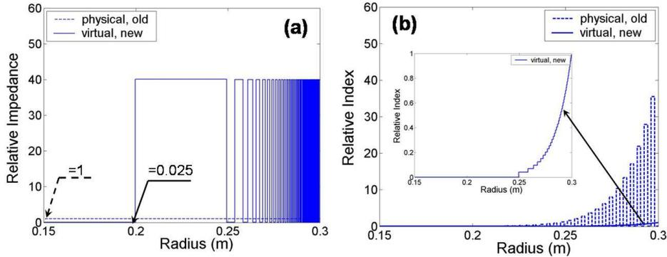
Fig. 8. The impedance (a) and index (b) profiles of  $x = 20$  isotropic cloaks for two cases: 1) the traditional *old* set when the ideal  $x = 20$  cloak is equally divided in “physical” space; 2) the current two-fold method
