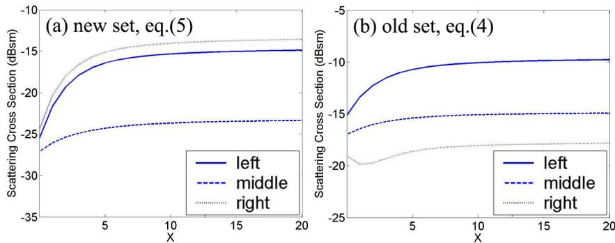
Fig. 3. The scattering cross section of the NTB spherical cloak versus the transformation nonlinearity, approximated by an isotropic non-ideal cloak. Three choices of positions (**L**, **M**, **R** in Fig. 2) under two sets of isotropic materials (a) *new* set and (b) *old* set are investigated and compared.
