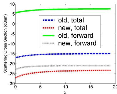
Fig. 5. Total and forward scattering cross sections for isotropic non-ideal cloaks designed by the *old* set (blue and green lines) and *new* set (red and black lines) versus the nonlinearity  $x$  in the coordinate transformation.
