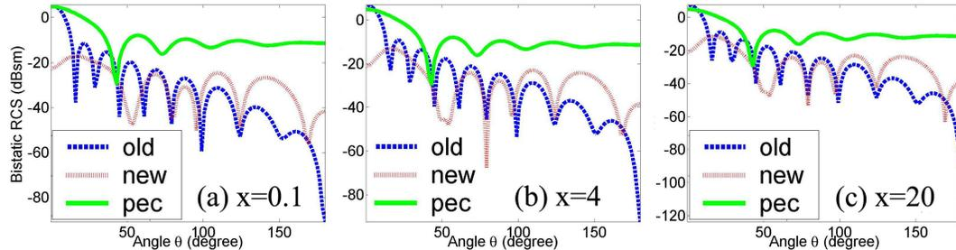
Fig. 4. Bistatic RCS for (a)  $x=0.1$ ; (b)  $x=4$ ; and (c)  $x=20$ . The RCS is normalized by  $\lambda_0^2$ , where  $\lambda_0$  denotes the wavelength in free space. The curves characterized by *old* and *new* correspond to the isotropic non-ideal cloaks designed by Eq. (4) and Eq. (5), respectively.
