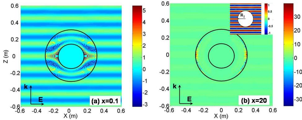
Fig. 6. The real part of  $E_x$  on the  $x$ - $z$  plane of the improved cloaks designed by *new* set for (a) $x=0.1$ ; (b)  $x=20$ . The inset in (b) only shows the total electric field outside the cloak (i.e.,  $r > R_2$ ) excluding the region in white ( $0 < r < R_2$ ). The working frequency is chosen to be 2GHz.
