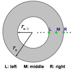
Fig. 2. The shadowed region denotes the  $n$ -th discretized anisotropic layer as in the upper-left illustration in Fig. 1. Before converting an discretized anisotropic layer into 2 isotropic sub-layers, we consider three positions generally (i.e., left  $\rightarrow r = r_{n-1}$ ; middle  $\rightarrow r = (r_{n-1} + r_n)/2$ ; right  $\rightarrow r = r_n$ ). In each case, this anisotropic layer's parameters, determined from Eq. (2), are uniform and constant within.
