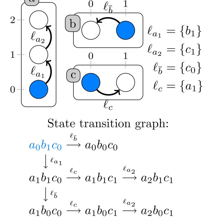
Asynchronous Automata Networks
