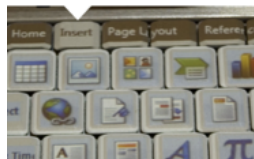
Figure 22: Command-hotkey mapping displayed on the keyboard. The TDK Keyboard [Block et al. 2010]. Icon are dynamically displayed on the corresponding hotkey, @ACM
