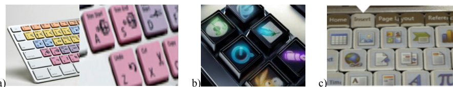
Figure 22: Command-hotkey mapping displayed on the keyboard. a) The logicKeyboard [LogicKeyboard] (b) the Optimus Keyboard [Optimus], (c) TDK Keyboard [Block et al. 2010]. An icon is statically (a) or dynamically (b,c) displayed on the corresponding hotkey.
