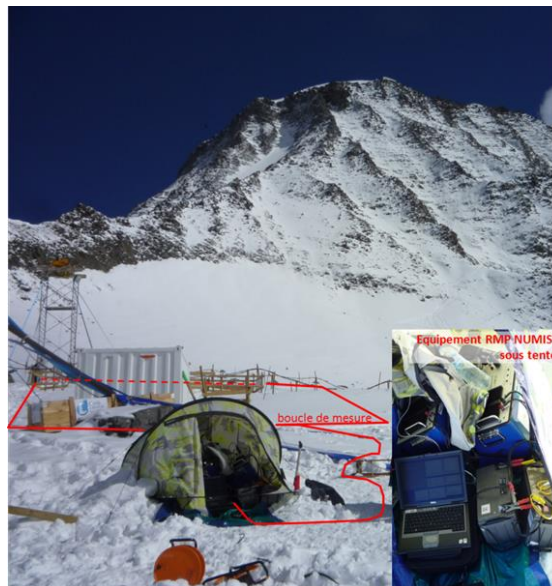
Fig. 1, The “Tete Rousse glacier” is located at 3200m altitude, the equipment is installed during 10 days in a tent, and the operators installed the 80x80 m loops generally on the snow.
