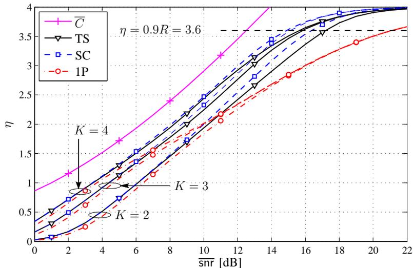
Fig. 2: Throughput of the proposed multi-packet HARQ TS and SC with  $T_p = 32$  are compared to the conventional HARQ 1P and the ergodic capacity  $\bar{C}$  when  $R = 4$  bits/channel use and  $K = 2, 3$  and  $4$ .
