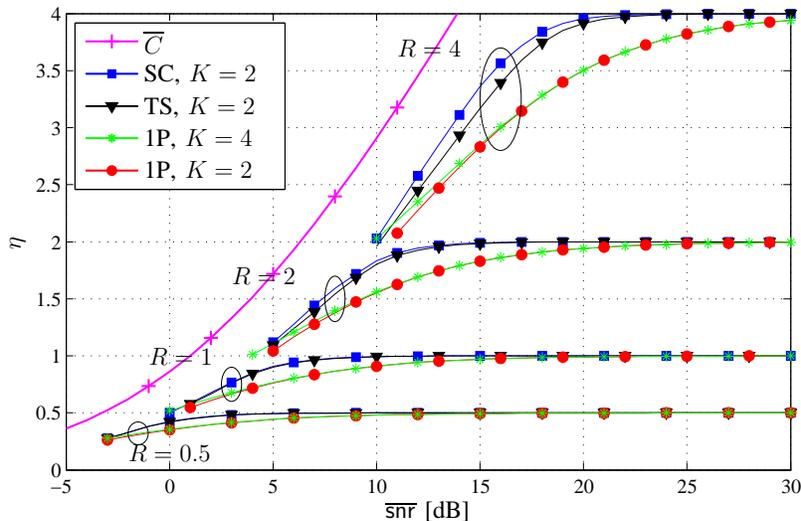
Fig. 6: Throughput obtained for various values of  $R$  bits/channel use, where for clarity, the results are shown only for  $\eta > R/2$ .
