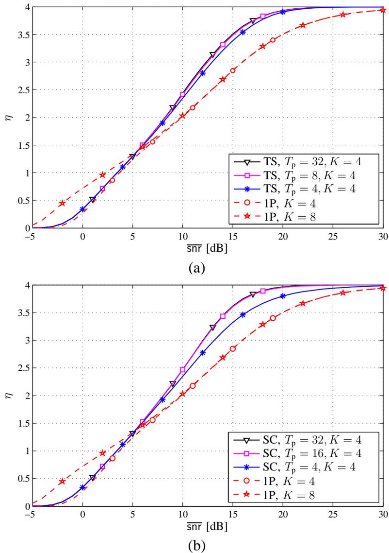
Fig. 7: Throughput of the proposed multi-packet in the case of (a) HARQ with TS and (b) HARQ with SC. Different values of  $T_p$  are considered and  $R = 4$  bits/channel use. The throughput of the conventional HARQ 1P is shown for comparison.
