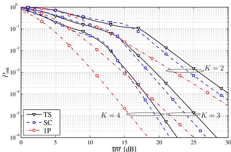
Fig. 4: Outage corresponding to the one-packet and multiple-packet HARQ when  $R = 4$  bits/channel use and  $T_p = 32$ .
