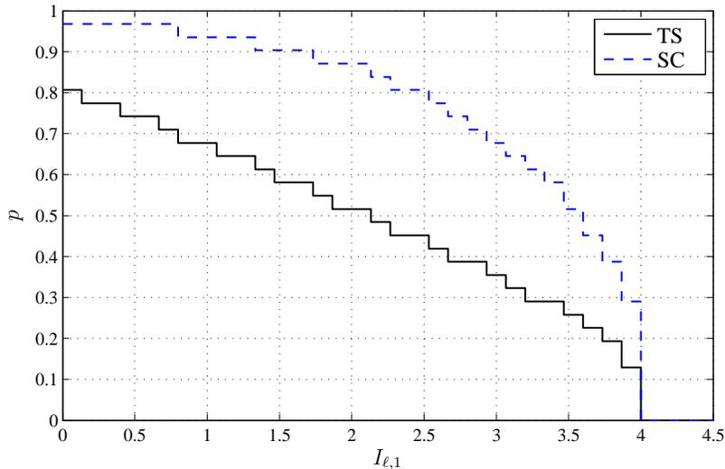
Fig. 5: An example of the optimal parameter  $p$  obtained for TS and SC when  $R = 4$  bits/channel use,  $\overline{\text{snr}} = 16$  dB,  $T_p = 32$  and  $K = 4$ .
