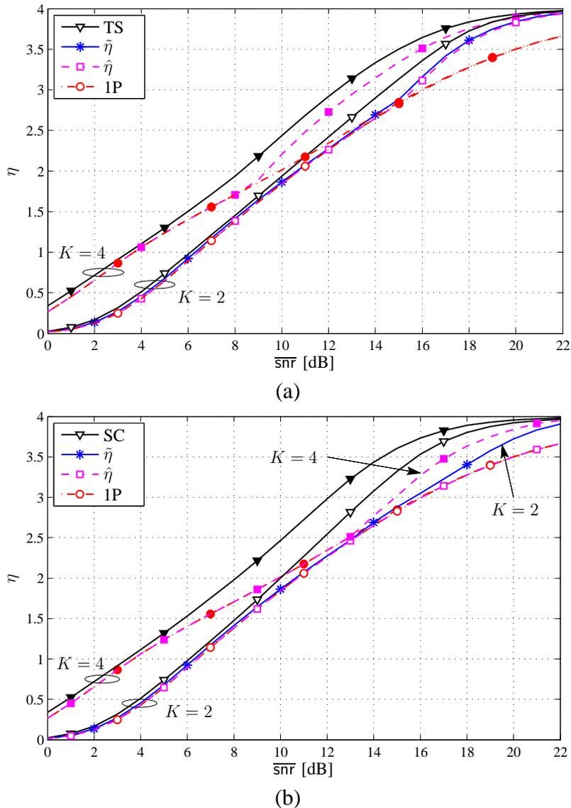
Fig. 8: Throughput of the multi-packet HARQ in the case of (a)  $\mathcal{A} = \mathcal{A}_{\text{mod}}^{\text{TS}} \times \mathcal{A}_p$  and (b)  $\mathcal{A} = \mathcal{A}_{\text{mod}}^{\text{SC}} \times \mathcal{A}_p$ ; the multi-bit feedback (TS), one-bit feedback ( $\tilde{\eta}$ ), unique-action one-bit feedback ( $\hat{\eta}$ ) and conventional one-packet HARQ (1P).  $T_p = 16$  and  $R = 4$  bits/channel use.
