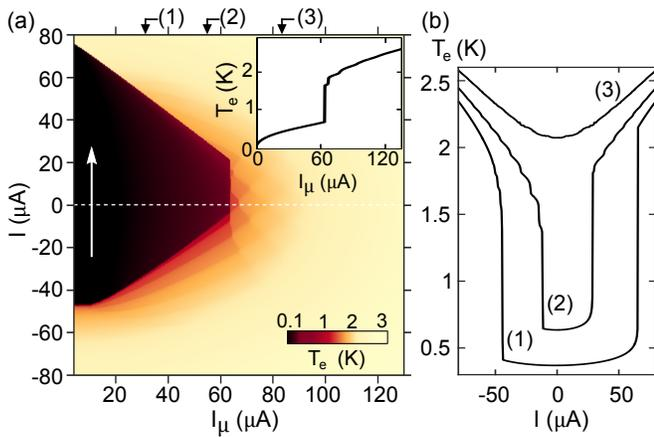
FIG. 3. (a) Calculated electronic temperature  $T_e$  map corresponding to situation of Fig. 2, i.e. for device J2 at  $T_{\text{bath}} = 100$  mK. Inset: Line cut showing the electronic temperature at zero dc bias current as a function of the microwave current. (b) Line cuts of the map (a) showing the dependence of the electronic temperature as a function of the dc bias current  $I$  at different values of the microwave current indicated by arrows at the top of the map.
