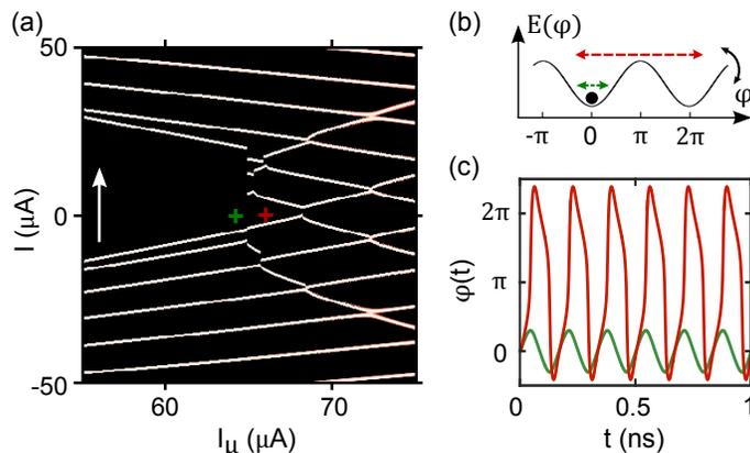
FIG. S1. (a) Zoom of the differential resistance map as a function of  $I$  and  $I_\mu$  at  $\nu = 6$  GHz (device J2,  $T_{bath} = 100$  mK) shown in Fig. 2e in the main paper. (b) Schematics showing the extent of the phase excursion at the two bias points. (c) Calculated time dependence of the phase at the bias points indicated by the crosses in (a).
