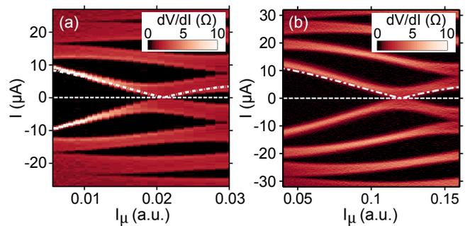
FIG. 4. a, b: Differential resistance maps as a function of  $I$  and  $I_\mu$  for  $\nu = 6$  GHz in non-hysteretic conditions, for (a) at base temperature and a magnetic field of 100 mT (device J2), and (b) at a bath temperature of about 4.2 K (device J3, no magnetic field). The white lines represent the usual Bessel-function-like amplitude of the step  $n = 0$ .
