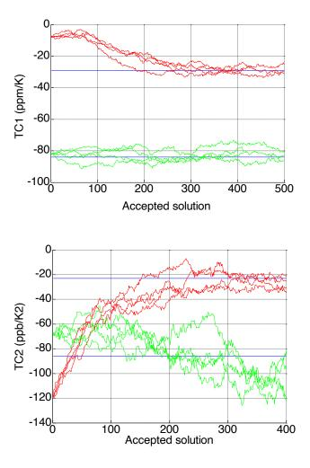
Fig. 5. Convergence paths for C66 (red) and C13 (green). Top: TC1 values; bottom: TC2 values. 'Accepted solution' refers to the number of new sets (**X**) accepted as solutions by the SA algorithm, during the optimization.
