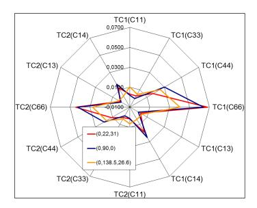
Fig. 6. Sensitivity map. Effect (ΔZ) of a +1ppm/K (+1ppb/K<sup>2</sup>) change of TC1 (TC2) values on the computed error Z.
