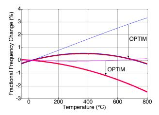
Fig. 12. Optimization from a distant starting point generated with  $\sigma = 35$ , for (0°, 22°, 31°) (above) and (0°, 138.5°, 26.6°) (below). Thin line(s): before optimization; Thick line(s): after optimization.
