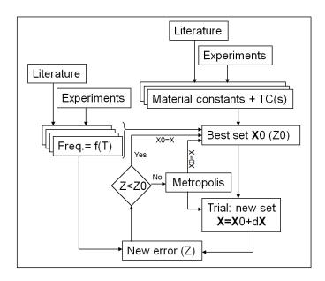
Fig. 1. The optimization procedure.
