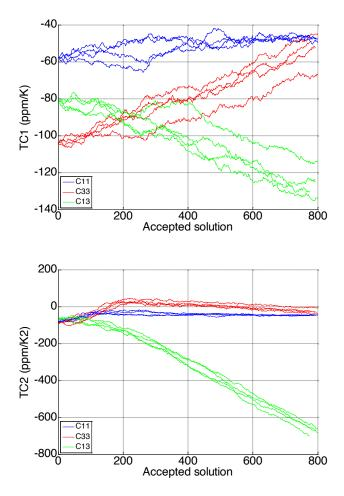
Fig. 9. Convergence patterns for C11, C33 and C31 when L-BAW and SAW curves are used as targets. Well-defined convergence patterns are visible for each of the coefficients. Top: TC1 values; bottom: TC2 values.
