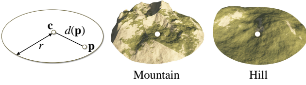
Figure 5: Disc primitives allow to generate landforms in small circular areas. Various elevation functions can be used: a constant function will represent a plain or plateau, a turbulence will produce hills and a ridge multi-fractals noise function [MKM89] will mimic mountains landscapes.
