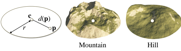
Figure 5: Disc primitives allow to generate landforms in small circular areas. Various elevation functions can be used: a constant function will represent a plain or plateau, a turbulence will produce hills and a ridge multi-fractals noise function [MKM89] will mimic mountains landscapes.
