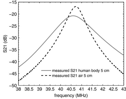
**Fig. 15.** Measured coupling response  $S_{21}$ , according to the frequency, between the capsule coil and the receiver coil separated by a distance of 5 cm when the path is the human body and the air.
