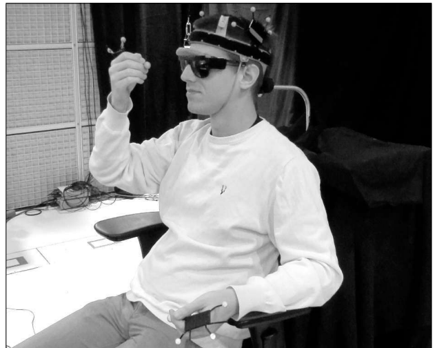
Figure 1. Photo of the proximal pointing task. The participant holds a rigid body in each hand, aligning the reference marker with his fingertips. The head is supported by a neck-rest to prevent head movements, and the head position and orientation were monitored in real-time using the motion capture system (inner frame of a helmet with reflective markers). The subjects were free to use the hand of their choice according to the most comfortable way to indicate the direction of the sound source, which is computed with regard to the current head position.
