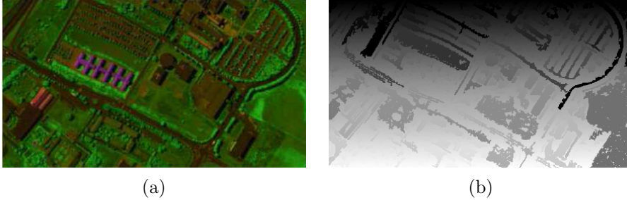
Figure 11: (a) A 3-variant image (first three eigenimages after PCA on Pavia hyperspectral image) and (b) its corresponding \alpha -flat zone partition into 84931 spatial classes using the Euclidean distance.
