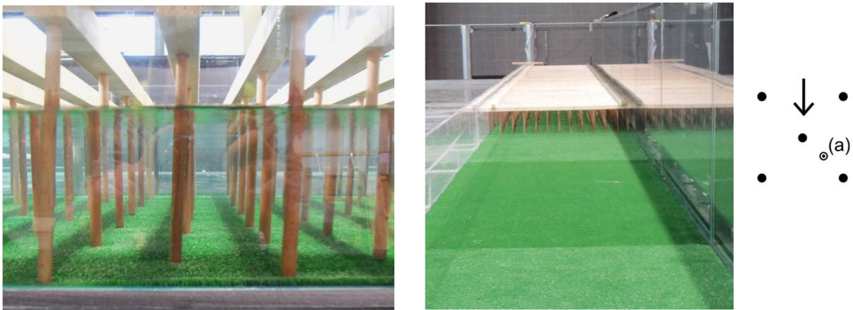
Figure 1: Left: Flow through staggered arrays of emergent rigid stems representing a wood; Middle: view from upstream of a meadow-to-wood transition; Right: position of measurement (a) within the array of stems.
