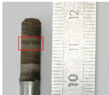
Fig. 4.7 Photography of the ore sample. The zone view by the X-ray tomograph is delimited by a red rectangle.
