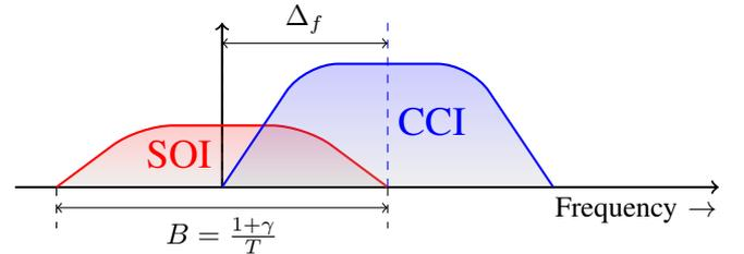
Fig. 2. Spectral representation of the SOI and CCI
