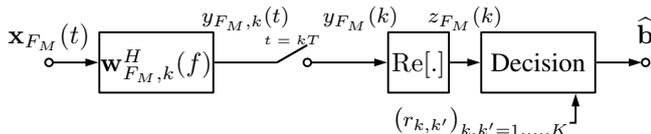
Fig. 1. Structure of the  $M$  input pseudo-MLSE receiver ( $M = 1, 2$ )
