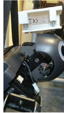
Fig. 2: GR1 detector attached to H@RI's head
