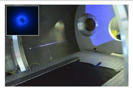
**Figure 1.** A photograph of the time-integrated fluorescence by the plasma column produced in air by a 10 J, 10 ps laser pulse, propagating from right to left and slightly downward. The inset shows fluorescence induced by the laser beam on a white paper screen placed in the far field. The dark area in the center of the image results from the screening of the trailing edge of the laser pulse by the dense and transversely uniform plasma channel.
