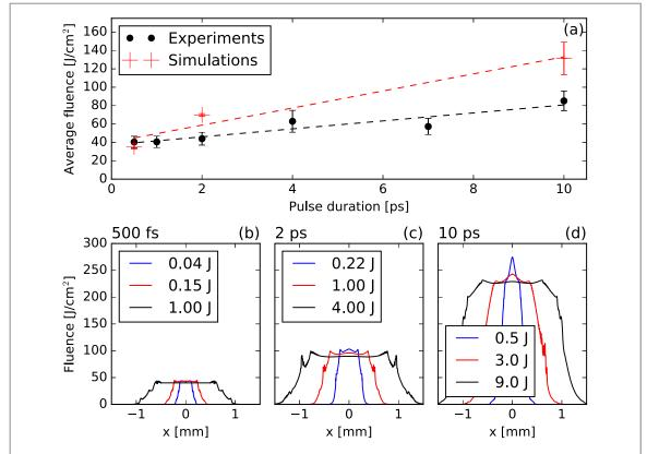
Figure 3. (a) Measured (•) and simulated (+) average laser fluence at the position of peak air ionization, versus pulse duration. At any given pulse duration, the average fluence is clamped, i.e., approximately independent of the pulse energy. Error bars are computed from deviations from the regression curves (i.e., see figure 2(a)). (b)–(d) Computed fluence profiles at the positions of peak ionization, for various pulse configurations, showing fluence clamping.
