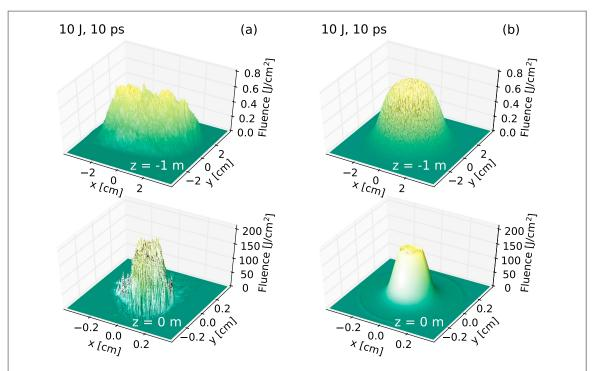
**Figure 5.** Fluence profiles computed using the time-integrated propagation model equation (10) and (a) a realistic noisy input beam and (b) a 4th order super-Gaussian input fluence profile perturbed by 10% amplitude random noise (see text for details). In both cases, the beam profiles 1 m before and at the linear focal plane are shown in the top and bottom panels, respectively.
