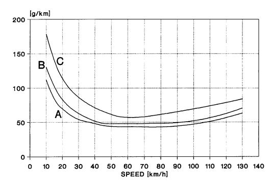
Figure VI.1.1-25: Speed-Dependent Fuel Consumption of Gasoline Vehicles < 2.5 t with a Cylinder Capacity < 1.4 l (A) and 1.4 - 2 l for the Sub-Category "Improved Conventional"
