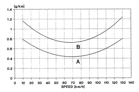
Figure VI.1.2-4: Speed-Dependent Particulate Emission Factors of Diesel Vehicles < 2.5 t Irrespective of Cylinder Capacity
