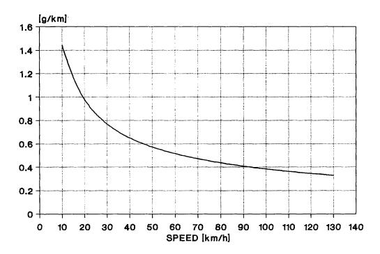
Figure VI.1.2-2: Speed-Dependent VOC Emission Factors of Diesel Vehicles <2.5 t Irrespective of Cylinder Capacity
