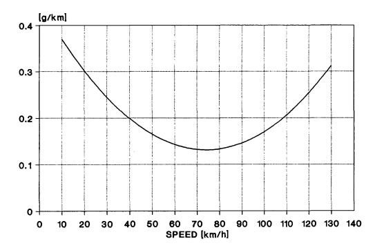
Figure VI.1.2-5: Speed-Dependent Fuel Consumption Factors of Diesel Vehicles <2.5 t
