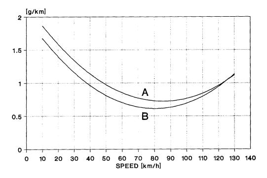
Figure VI.1.1-17: Speed-Dependent VOC Emission Factors of Gasoline Vehicles <2.5 t with a Cylinder Capacity of <1.4 l (A) and 1.4 - 2.0 l (B) for the Sub-Category "Open Loop"
