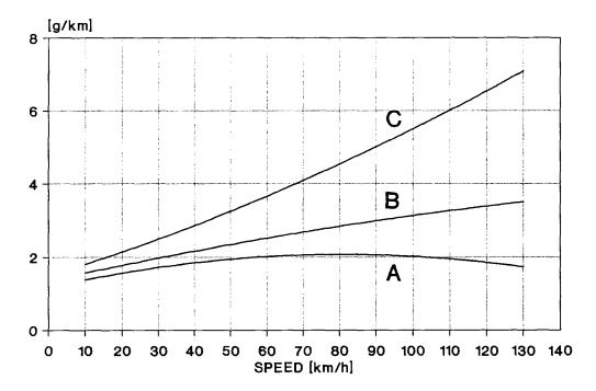
Figure VI.1.1-11: Speed-Dependent NOx Emission Factor of Gasoline Vehicles <2.5 t for ECE 15-02 Homologation and Vehicles with Cylinder Capacity <1.41(A), 1.4-21(B) and >21(C)
