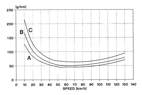
Figure VI.1.1-24: Speed-Dependent Fuel Consumption of Gasoline Vehicles < 2.5 t for ECE 15-04 Homologation and Vehicles with Cylinder Capacity < 1.4 l (A), 1.4 - 2 l (B) and > 2 l (C)
