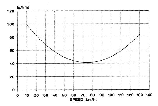
Figure VI.1.3-1: Speed-Dependent CO Emission Factors of LPG Vehicles <2.5 t
