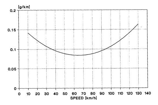
Figure VI.1.1-20 (cont.): Speed-Dependent NOx Emission Factors of Gasoline Vehicles <2.5t irrespective of Cylinder Capacity for the Sub-Category "Closed Loop"
