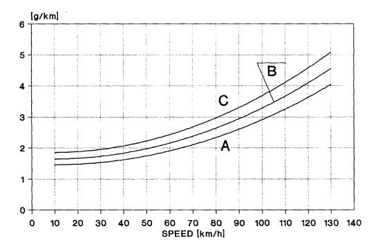
Figure VI.1.1-12: Speed-Dependent NOx Emission Factor of Gasoline Vehicles <2.5 t for ECE 15-03 Homologation and Vehicles with Cylinder Capacity <1.41(A), 1.4-21(B) and >21(C)
