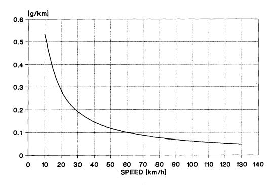
Figure VI.1.2-3: Speed-Dependent NOx Emission Factors of Diesel Vehicles < 2.5 t with a Capacity of < 2.0 l (A) and > 2.0 l (B)
