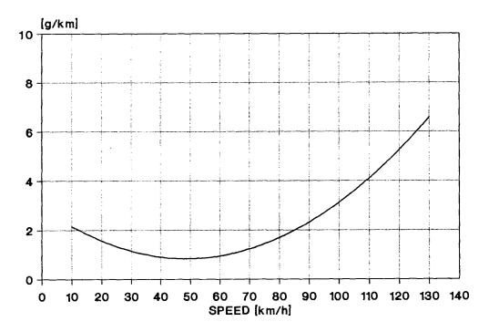
Figure VI.1.1-20 (cont.): Speed-Dependent VOC Emission Factors of Gasoline Vehicles <2.5t irrespective of Cylinder Capacity for the Sub-Category "Closed Loop"
