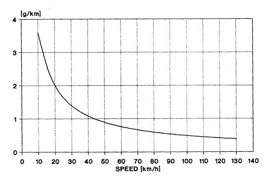
Figure VI.1.3-3: Speed-Dependent NOx Emission Factors of LPG Vehicles < 2.5 t
