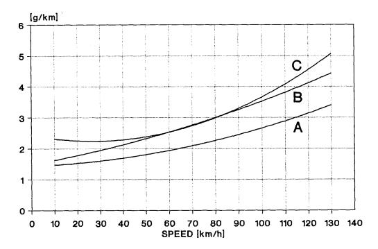
Figure VI.1.1-14: Speed-Dependent CO Emission Factors of Gasoline Vehicles <2.5 t with a Cylinder Capacity <1.4 l (A) and 1.4 - 2 l (B) for the Sub-Category "Improved Conventional"
