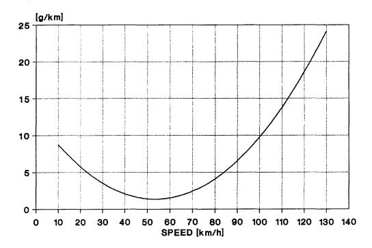
Figure VI.1.3-2: Speed-Dependent VOC Emission Factors of LPG Vehicles < 2.5 t
