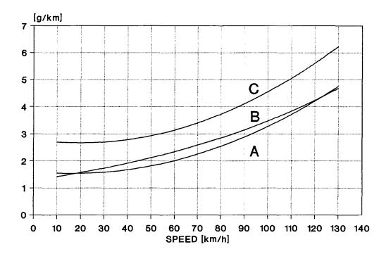
Figure VI.1.1-13: Speed-Dependent NOx Emission Factor of Gasoline Vehicles <2.5 t for ECE 15-04 Homologation and Vehicles with Cylinder Capacity <1.41(A), 1.4 - 21(B) and >21(C)
