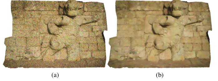
Figure 4: Filtering of a noisy Maya wall with preservation of edges, (a) noisy point cloud, (b) denoised point cloud.
