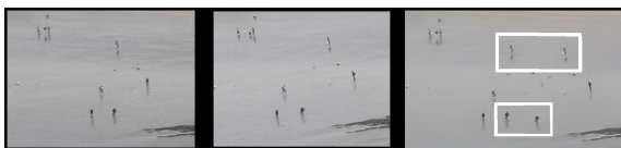
Figure 3: From left to right, a zoom on two images to be stitched, and the assembling error with double occurrences of humans (highlighted with white frames).
