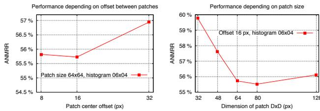
Fig. 2. Experiments for choosing the patch size and offset between patches. The tuning was done using smaller descriptors, with histograms of dimensions  $6 \times 4$  and histograms size 48, while the chosen patch size ( $80 \times 80$ ) and offset between patches (16 pixels, resulting in 64 pixels of overlap for the chosen patch size) are later used with a larger histogram sizes.
