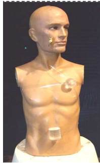
FIG. 12: Mannequin with 2 low permittivity explosives simulants.
