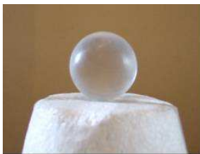
FIG. 14 : Dielectric sphere ( \epsilon_r=2.53 , D=50.8\text{mm} )
