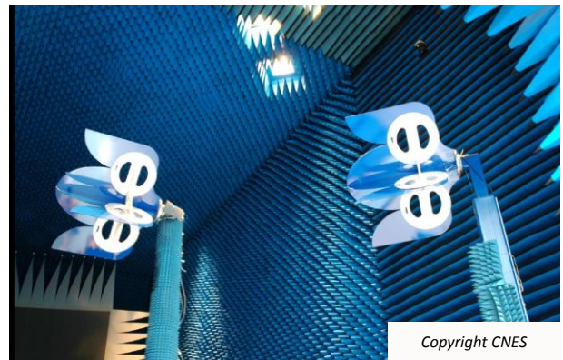
Figure 1 Photograph of the dual polarized probe in the CNES VHF Near-Field system
