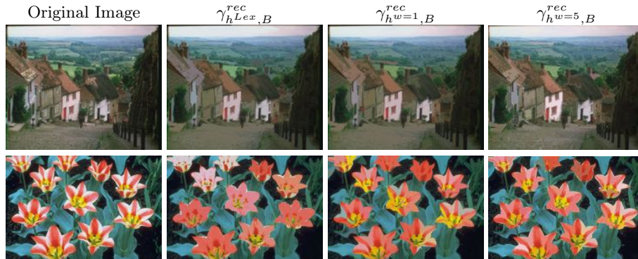
Fig. 2. Opening by reconstruction of color images by lexicographic color lattice ( h^{Lex} ) or learned complete lattice from color ( h^{w=1} ) and 5 \times 5 patches ( h^{w=5} ). The marker image is obtained from an erosion in the same lattice with a square structuring element of side 11 pixels.
