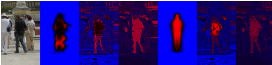
Fig. 4. Example of probability map estimation. From left to right: initial image, appearance based probabilities, color histogram based probabilities from appearance based probabilities, Color GMM based probabilities from appearance based probabilities, shape template prior based probabilities, color histogram based probabilities from shape template prior based probabilities and GMM based probabilities from shape template prior based probabilities.
